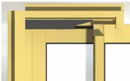
Tapered sash buffer stop to keep panel on the track.
